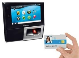
Figure 335: Authentication with user's BIOPIN on contactless card
