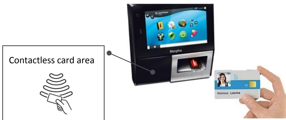
Figure 338: Authentication without biometric check and with User ID check in card
