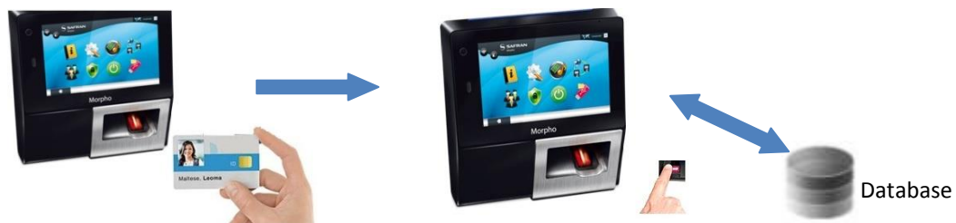
Figure 336: Authentication with biometric check, reference in database
