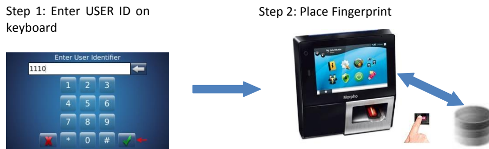
Figure 337: Authentication with User ID entered from Keyboard and biometric check
