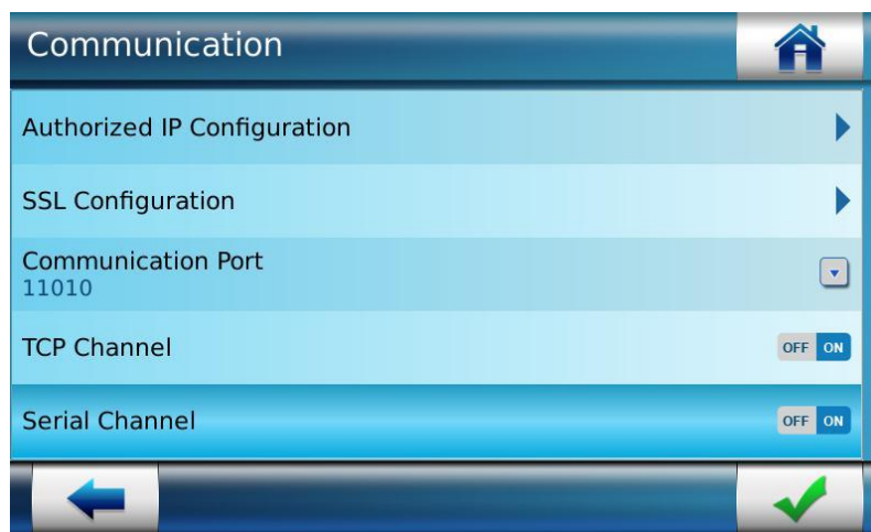
Figure 221: Enabling/Disabling RS422/RS485 Serial Chanel
